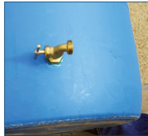
Figure 18. Hose bib facing to the side.
